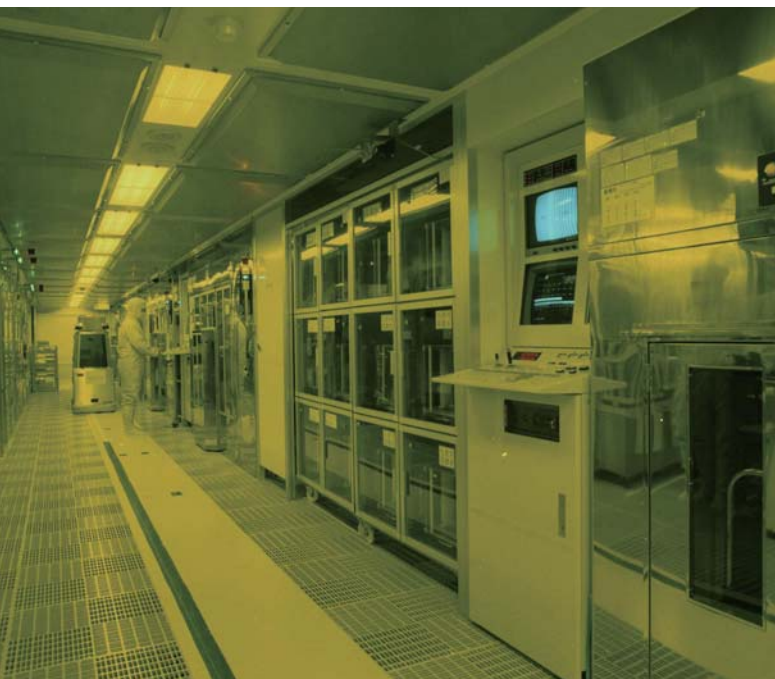
Microfabrication processing line for color TFT LCDs (Tenri Plant)
